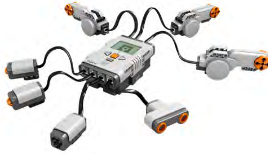
Figure 4.1.: The Programmable Brick Computer with Motors and Sensors Attached (cf. Lego.com [Leg13])
