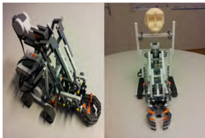
Fig. 2: The functional and the more human-like robot with a 3D printed head following the model of Neophyte.
