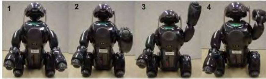
Figure 3.4.: Possible Postures for each Foreleg of the AIBO Robot (cf. Guo [GS08], S. 6)
