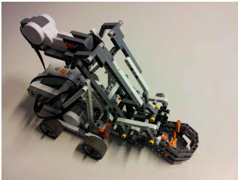
Figure 4.3.: The Functional Prototype with the Grabbing Arm
