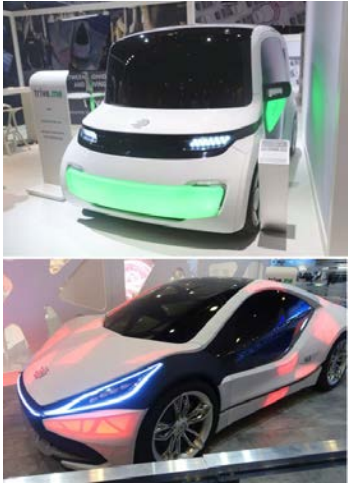
Figure 2: Vehicle prototypes communicating information through light embedded in the vehicle body. Frankfurt Motor Show, IAA'15. Taken by authors. http://trive.me
