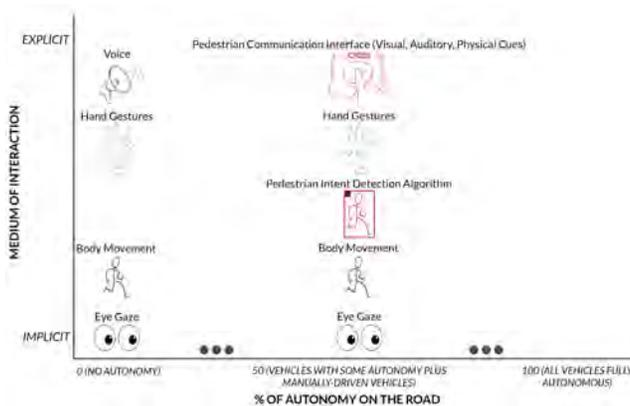
**Figure 2:** Mediums of interaction that a pedestrian can use for vehicles with different levels of autonomous behavior.
