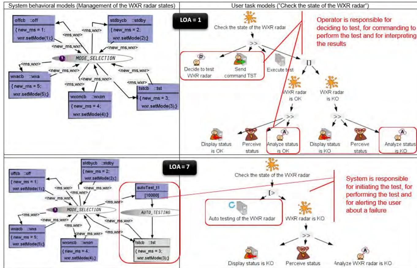
**Figure 1:** Two versions of the models of the system behavior and of the user tasks for function "Check the state of the WXR radar" (two different automation levels according to the classification of Parasuraman [13])
